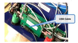
b) The Control Board connectors are locked by **small black wire ties**, one at each end; **clip** these wire ties free (note attachment method for re-connecting)
