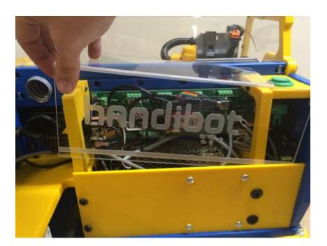
Secure cover in place using red handled hex key.
