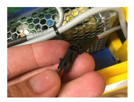
Make sure that the ribbon cable is plugged into the 16 pin header on the FabMo card in the orientation shown below.
