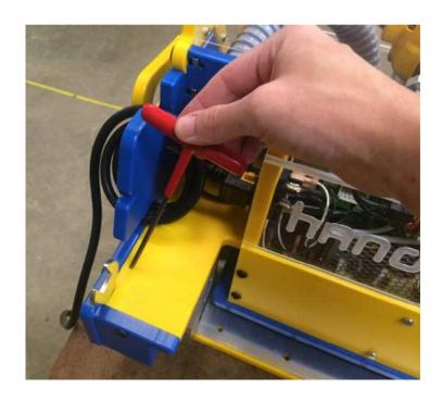
Remove the button head screw from the left, top side of the clear electronics enclosure.
