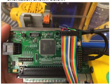
Plug the FabMo card into the interface board. The new Right-angle mount does not require mounting screws (retained by enclosure).
