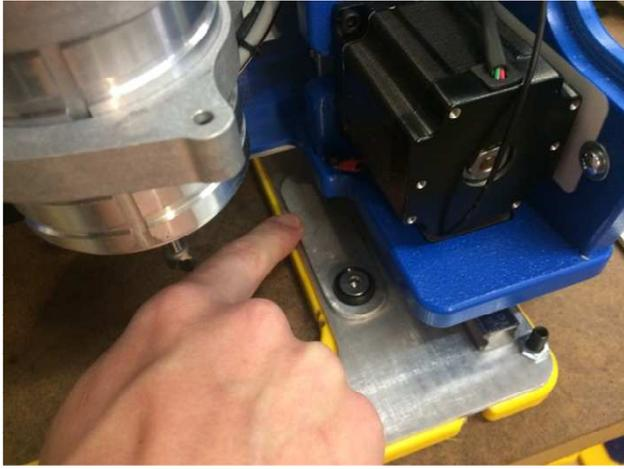
**13** Clip vacuum foot back onto router bracket.
